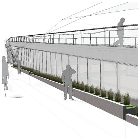
A bioretention planter treats polluted runoff generated from the alley
